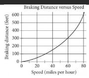
The graph above shows the relationship between the speed of a particular car, in miles per hour, and its corresponding braking distance, in feet. Approximately how many feet greater will the car's braking distance be when the car is traveling at 50 miles per hour than when the car is traveling at 30 miles per hour?
