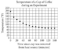
In an experiment, a heated cup of coffee is removed from a heat source, and the cup of coffee is then left in a room that is kept at a constant temperature. The graph above shows the temperature, in degrees Fahrenheit (°F), of the coffee immediately after being removed from the heat source and at 10-minute intervals thereafter. During which of the following 10-minute intervals does the temperature of the coffee decrease at the greatest average rate?
